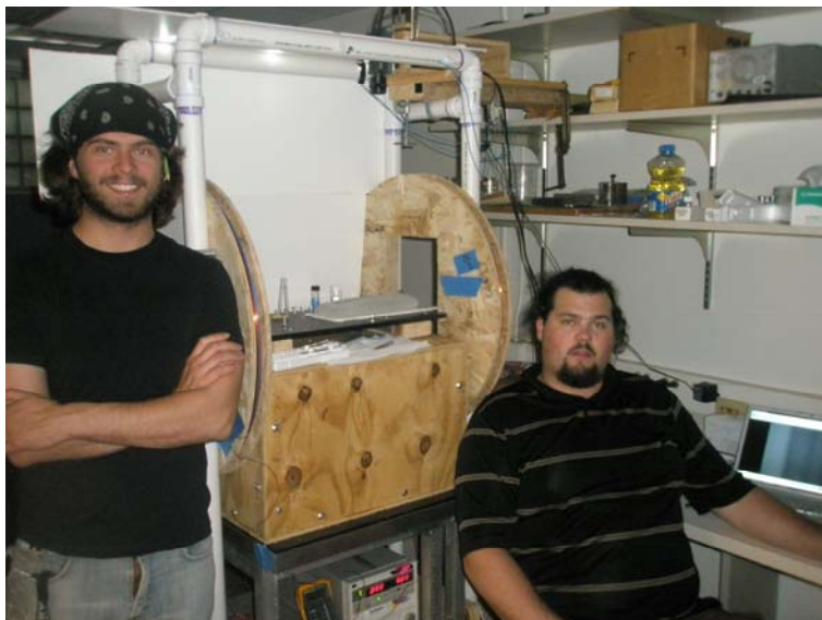
Figure 4 Student Researchers: Undergraduates Tom Lopez and Nate Johnson have made a prototype of a magnetic needle viscometer. The camera purchased with the SPS undergraduate award can be incorporated into an existing Labview program so image acquisition, instrument control, and data analysis can now be fully automated and done in one program.
