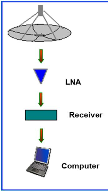
Figure 3 Radio telescope basic components [11].
