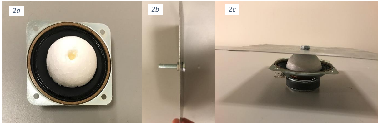
Figure 2 Set up of the Chladni plate on a speaker. Left: Top view without metal sheet. Middle: Side view of metal plate, nut, and bolt. Right: Speaker/foam assembly attached to the metal plate/bolt.
