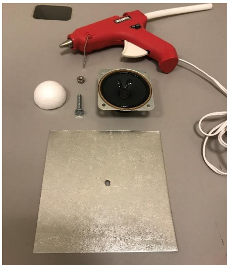
Figure 1 Materials for setting up the speaker version of the Chladni plate. Not pictured is the input mechanism (phone or frequency generator), amplifier, and sand.
