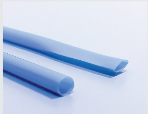
FIGURE 1: The original straw (left) and the flattened straw (right).
