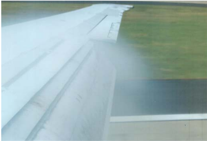
Fig. 7. Humidity making the flow visible. The condensation above the wing shows the pressure to be lower there.
