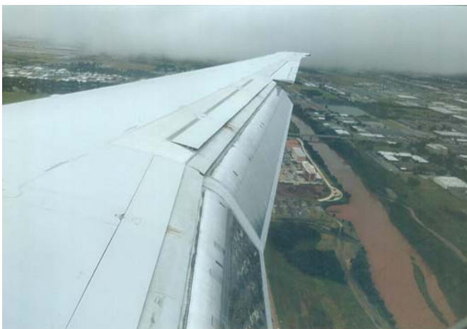
Fig. 6. Wing with flaps down deflecting the air's momentum.
