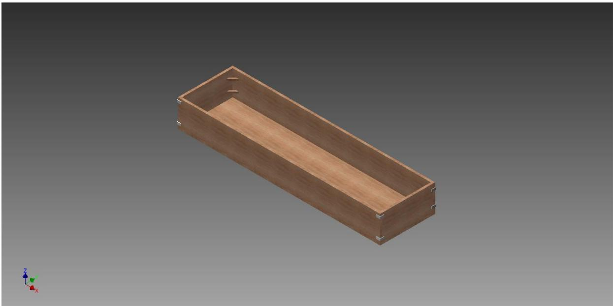
**This is a CAD drawing of the oobleck pool. A tarp would line the inside of the pool in order to hold the oobleck, and the edges of the tarp would be pinned beneath the pool.**
