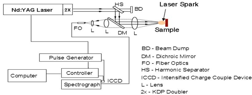
**Figure 1: Experimental set-up to obtain the LIBS spectra.**
