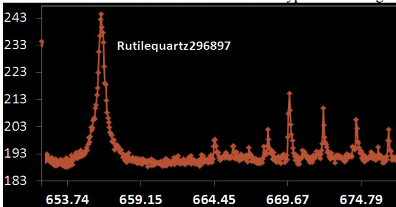
**Figure 2: LIBS spectrum of quartz.**
