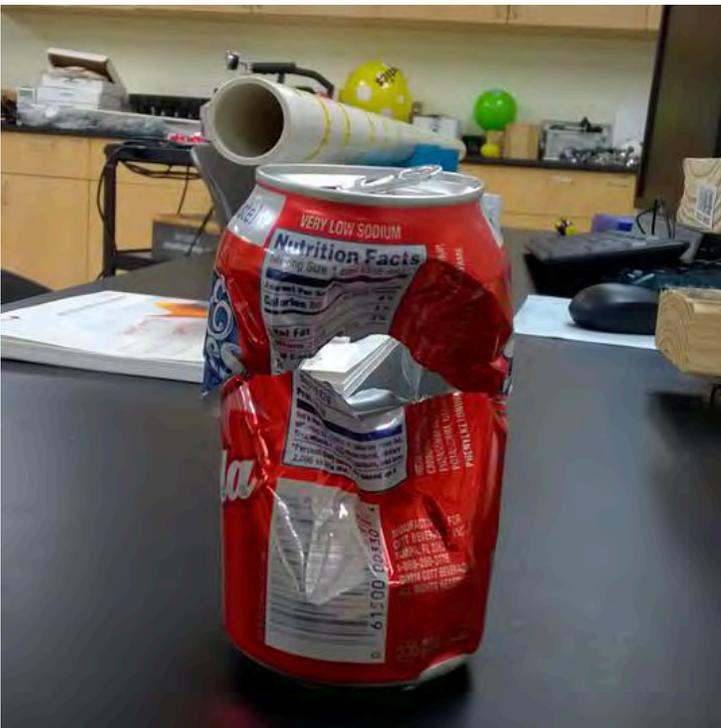
A close up shot of a soda can that was destroyed by the ping pong ball projectile launched by the TLU SPS Vacuum cannon. This was the can that produced the dangerous shrapnel piece.
