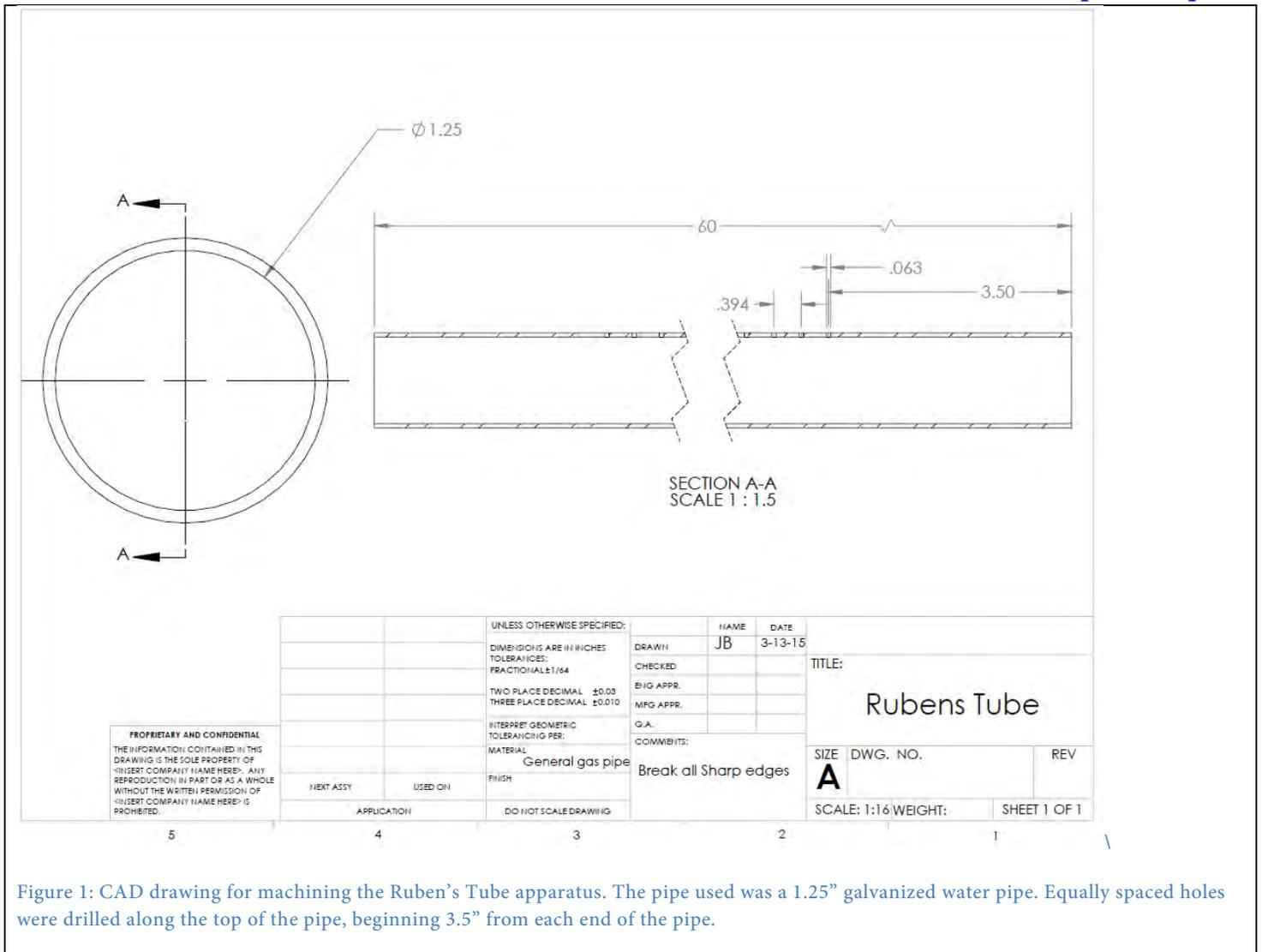
Figure 1: CAD drawing for machining the Ruben's Tube apparatus. The pipe used was a 1.25" galvanized water pipe. Equally spaced holes were drilled along the top of the pipe, beginning 3.5" from each end of the pipe.
