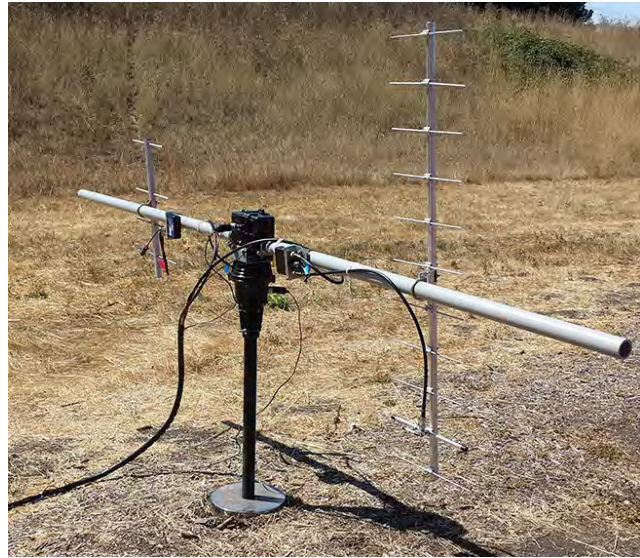
Temporary ground station mast, Yaesu G-5500 rotator and 70cm yagi antenna assemblies
