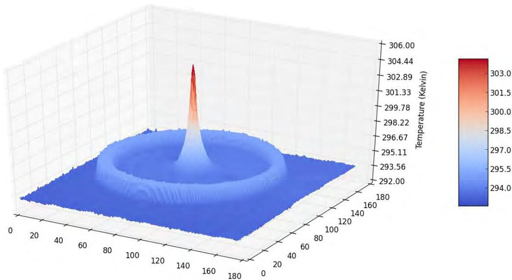
**Fig. 2** Plot of spatial variation of temperature of circular oil drop heated centrally with a laser pointer of 405 nm.
