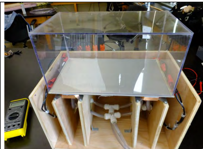
Figure 4: The chamber and aluminum plate resting on the cooling system.
