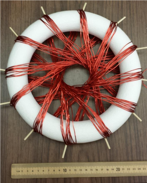
Figure 3. The “Medium” prototype consisting of twelve loops and ten winds of 16 AWG wire. The outer diameter of the torus measures 26 cm.
