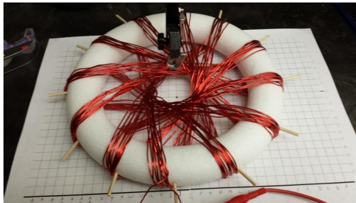
Figure 10. The set-up of the Gaussmeter probe held in place above the torus and grid. The torus is moved along the grid, simulating the movement of the probe, without interfering with the orientation or position of the probe.
