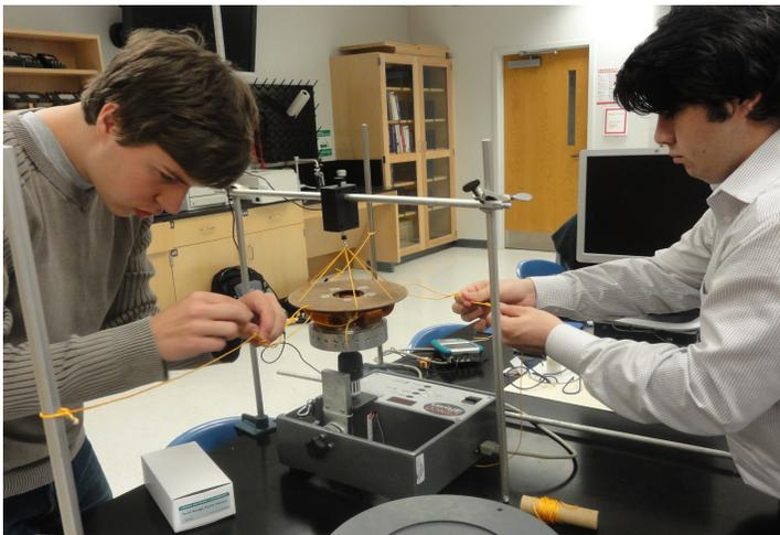
Austin and Ricardo experiment on rotating circular Halbach array - they measure a repulsive magnetic force on a coil system suspended on a force sensor.
