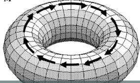
Torus with azimuthal magnetization ( $\vec{M}$ )
