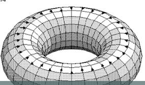
Toroidal coil with current density ( $\vec{J}_m$ )
