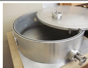
Test Vacuum Chamber
