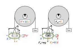
Fig. 2. Watt balance. Left: velocity mode. The coil moves vertically in a radial magnetic field, and a voltage V is induced. Right: force mode. The upward electromagnetic force generated by the coil opposes the gravitational force exerted on m. [4].
