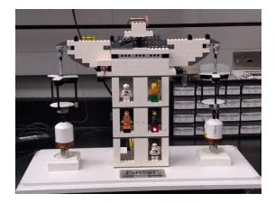
Fig. 4. The LEGO watt balance [4].
