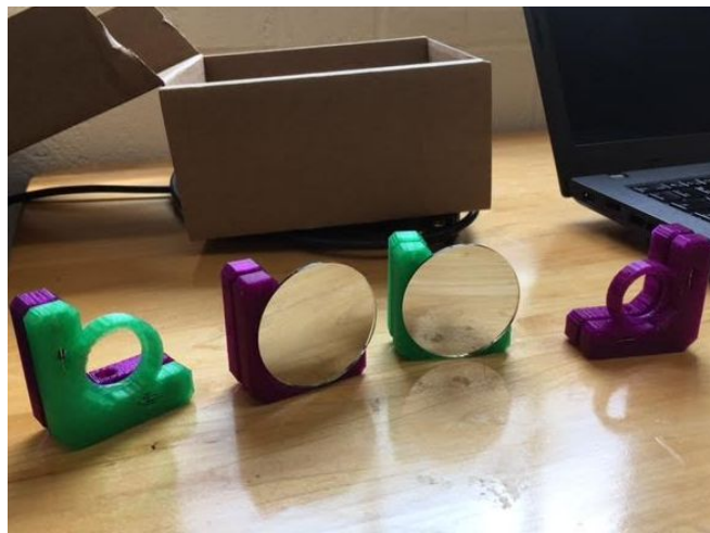
Figure 4: Mirrors and 3D printed optical mounts Taken By: John Evans
