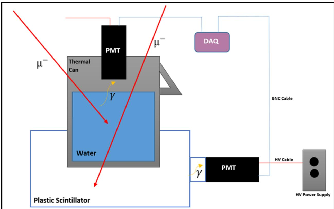
Figure 1. Diagram of the detector
