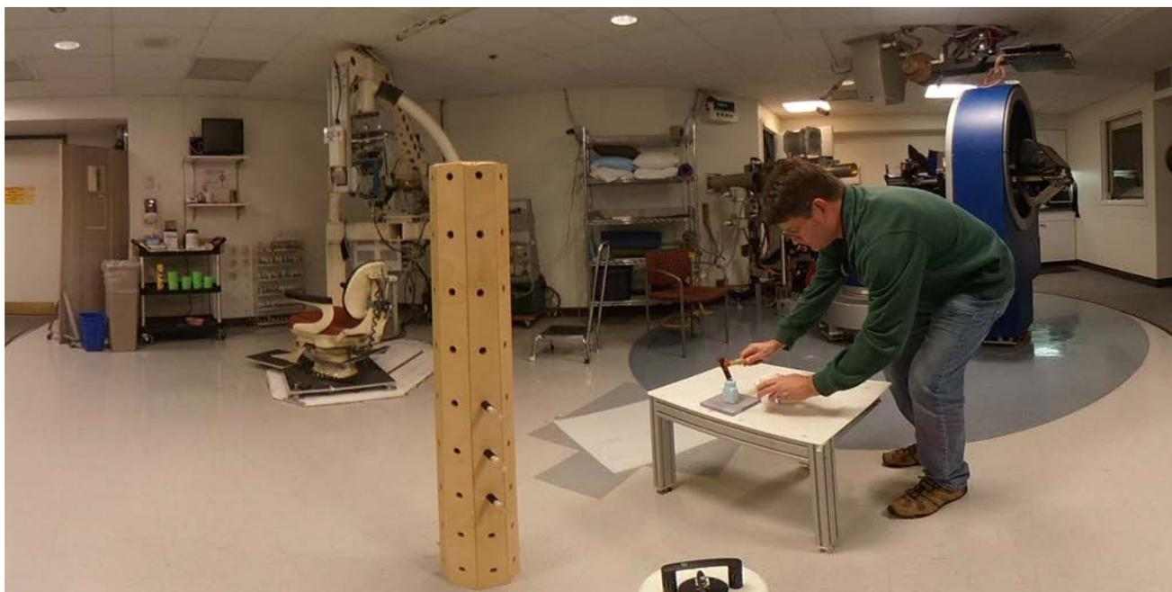
The neutron bubble detectors will be placed in a wooden stand that has 72 possible positions which was built by SPS and senior students John Thomas and Jackson Nolan, can be placed in any position, with respect to the AmBe source and the LINAC. In the above photos the array can be mounted on tripods as well as stand on its own. This array will be used to first measure a  $1/r^2$  dependence after which it can have the
