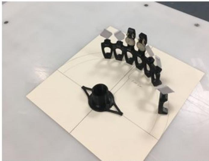
Figure 2 AmBe source array, foil order left to right; In-B, Au-F, In-A with Cd cover, Au-E with Cd cover, Dy-J, W-M, and In-C
