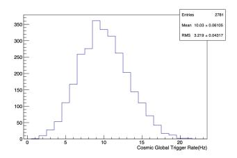
**FIGURE 8.** Global cosmic trigger rate had been continually measured by a VME scaler module from CAEN. The global coincidence trigger rate, of six top and six bottom scintillators, found to be (10.05 + /- 3.124) Hz matching the simulation value that is of 10.45 Hz. The distance between top and bottom scintillators is 19.2 cm.
