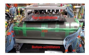
**FIGURE 6.** A view of the cosmic trigger system surrounding VXD, where the top scintillators are seen. The VXD is the sealed tube in the middle.
