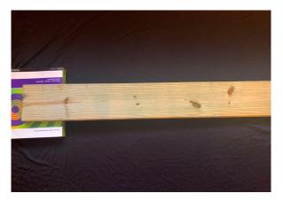
Figure 1: A board placed on a book to create an incline. An angle of  $10-20^{\circ}$  provides a reasonable time to measure for a board of ~1 m in length.
