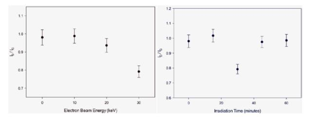
**FIGURE 3.** (a) Raman D- to G-band peak-intensity ratios (I<sub>D</sub>/I<sub>G</sub>) for GO samples irradiated for 30 minutes using 10 keV, 20 keV, and 30 keV electron beams. The data point at 0 keV corresponds to an as-purchased (unirradiated) GO sample. (b) Raman D- to G-band peak-intensity ratios (I<sub>D</sub>/I<sub>G</sub>) for GO samples irradiated using a 30 keV beam for 0, 15, 30, 45, and 60 minutes.
