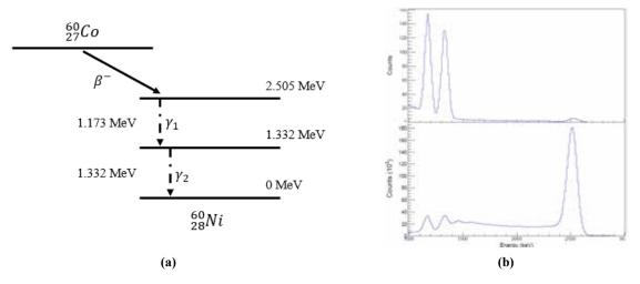
**FIGURE 2.** (a) Decay scheme for <sup>60</sup>Co. (b) TOP – single  $\gamma$ -ray spectrum. BOTTOM –  $\gamma$ -ray summation peak.
