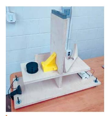
ABOVE: The prototype components: wood frame, pivot mount (gray), coil housing (black), support piece for the nylon guides (yellow), balance wheel and razor-blade pivot (resting upside down on the right side of the wooden frame), webcam (far left), and data acquisition device (far right). Photo courtesy of John Evans.
