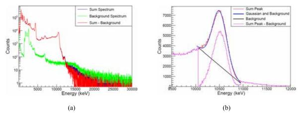
FIGURE 3. (a) Full γ-ray sum spectrum for a 6352.2 keV beam energy. Each colored line represents the following: original sum spectrum (blue), background spectrum (green), and sum spectrum after background subtraction (red). (b) Sum peak of the spectrum. Each colored line represents the following: original sum peak (red), Gaussian and first-order polynomial background fit (blue), background fit (black), and sum peak with background subtracted (purple).
