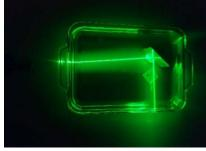
Figure 8. Laser beam going through the gelatin and reflecting off the mirror
