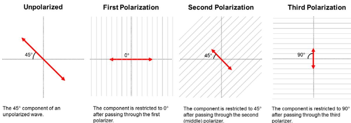
Once again, we examine a single plane of oscillation at  $45^\circ$ . After passing through the first polarizer, the vertical components are restricted and only the horizontal components pass through.
