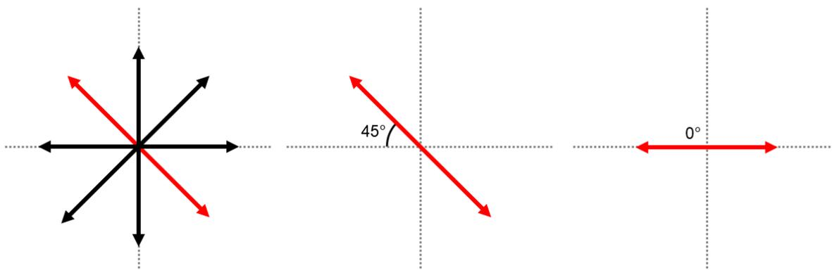
Figure 3: A single plane of oscillation (in red) passing through a polarizer which removes the vertical component. Only the horizontal component remains and the magnitude is decreased.
