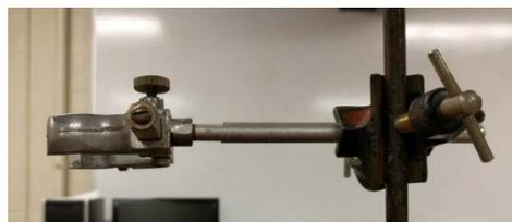
Figure 3: Extension clamp (slide-ended)
