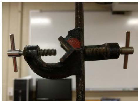
Figure 2: Double-ended bosshead clamp
