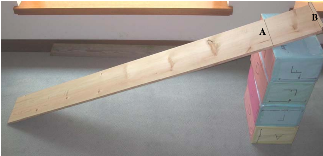
Figure 2 ó The ramp setup. A) Line used to align ramp with boxes. B) Wooden lip to align wheels of dynamics cart.
