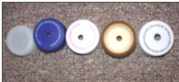
Figure 3 ó Picture of bottle caps with various sized holes drilled into them for nozzle optimization test.
