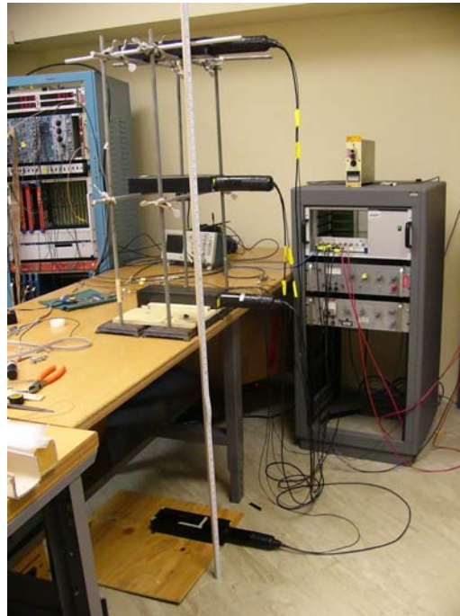
Figure 7. Experimental setup for the muon speed measurement.
