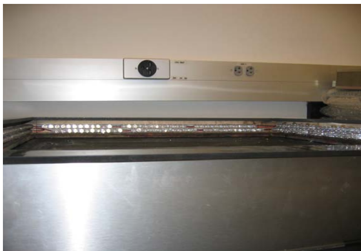
Figure 2 A photograph of the light strip constructed with 1cm LEDs and bread boards.
