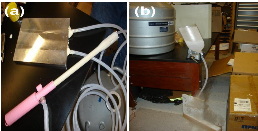
Figure 13 (a) Solid Al cold plate and a pump (b) An experimental setup that utilized gravitational force to supply LN2 into the cold plate
