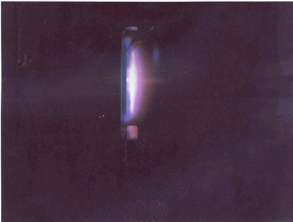
Figure 3: A picture of the plasma source in operation, taken through a side window of the vacuum chamber. Notice the narrow pink jet of plasma extending from the very center of the source.
