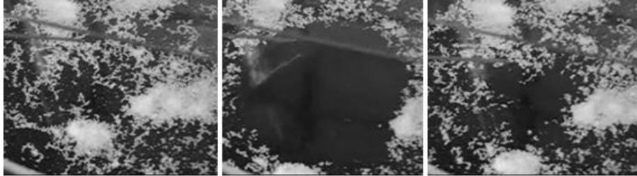
Fig. 1 From left to right: 1) Initial configuration of surface at time 0.0s. 2) Effect of solvent drop on surface at time = 0.4s. 3) Recovery of surface at time = 1.5s[3].
