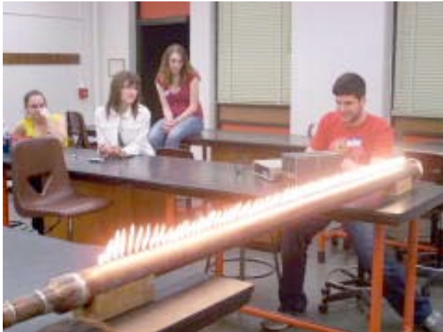
UC Davis' Rubens Tube and students are above. Dark photo Below shows clear uniform wavelengths.
