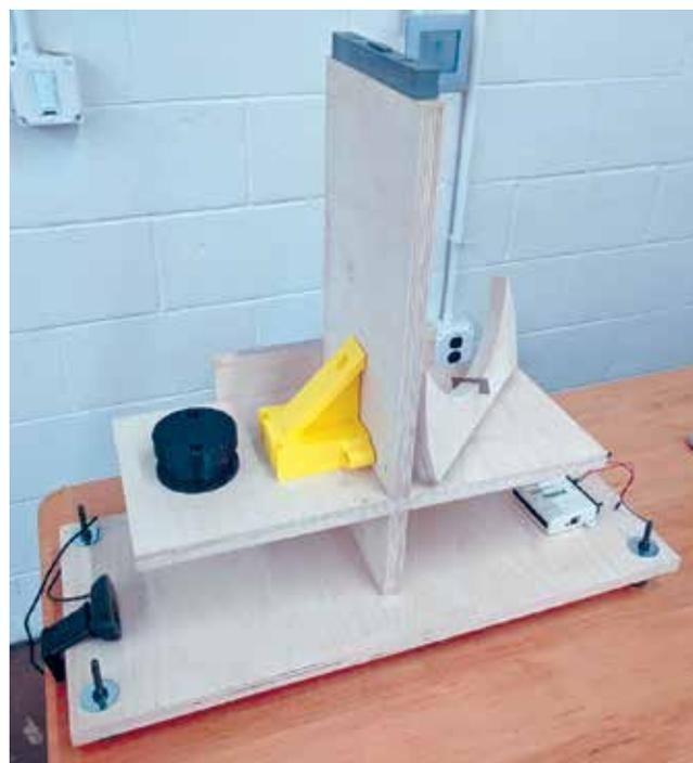
**ABOVE:** The prototype components: wood frame, pivot mount (gray), coil housing (black), support piece for the nylon guides (yellow), balance wheel and razor-blade pivot (resting upside down on the right side of the wooden frame), webcam (far left), and data acquisition device (far right). Photo courtesy of John Evans.
