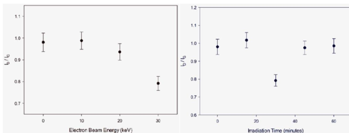
**FIGURE 3.** (a) Raman D- to G-band peak-intensity ratios ( $I_D/I_G$ ) for GO samples irradiated for 30 minutes using 10 keV, 20 keV, and 30 keV electron beams. The data point at 0 keV corresponds to an as-purchased (unirradiated) GO sample. (b) Raman D- to G-band peak-intensity ratios ( $I_D/I_G$ ) for GO samples irradiated using a 30 keV beam for 0, 15, 30, 45, and 60 minutes.
