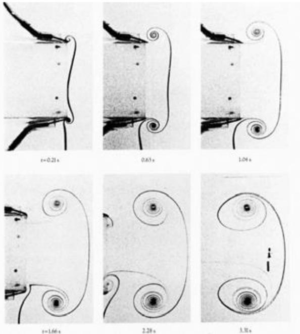
Figure 2. Formation of a vortex ring from a nozzle ejecting water
