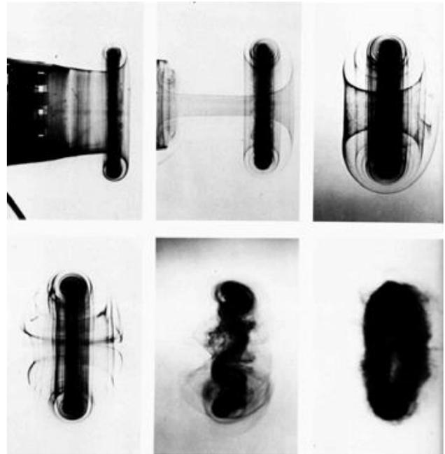
Figure 3. Step-by-step formation of a vortex ring from the moment the fluid is ejected to the formation of the ring
