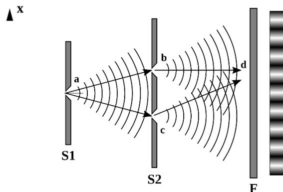
Figure 2: Diffraction pattern of two identical sources. By en:User:Lacatosias, User:Stannered (Image:Ebohr1.png) [GFDL (<http://www.gnu.org/copyleft/fdl.html>) or CC-BY-SA-3.0 (<http://creativecommons.org/licenses/by-sa/3.0/>)], via Wikimedia Commons
