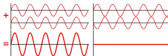
Figure 1: Constructive (Left) and Destructive (Right) linear superposition of waves. Modified from: original version: Haade; vectorization: Wjh31, Quibik (Vectorized from File:Interference of two waves.png) [CC BY-SA 3.0 (<http://creativecommons.org/licenses/by-sa/3.0>) or GFDL (<http://www.gnu.org/copyleft/fdl.html>)], via Wikimedia Commons
