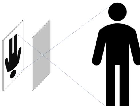
Instruct participants remove an 8 cm x 8 cm square from the center of their board. Cover the opening with aluminum foil and secure with tape. Next, gently pierce the foil in the center with a thumbtack. A small hole is desired: smaller holes will be dimmer, but have sharper focus. Collect thumbtacks after everyone has made their pinhole.
